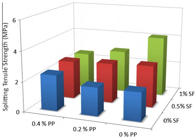
Fig. 4. Effect of steel and PP fiber on splitting tensile strength.
