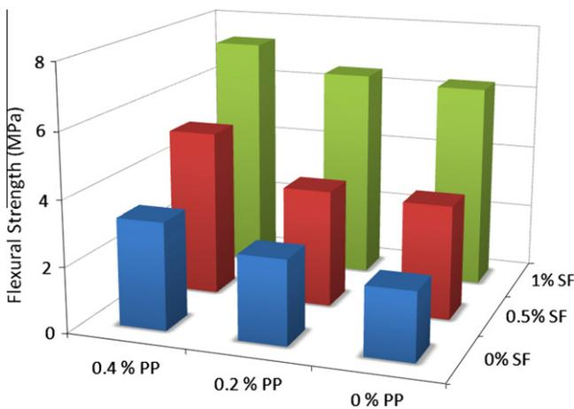
Fig. 3. Effect of steel and PP fiber on flexural strength.
