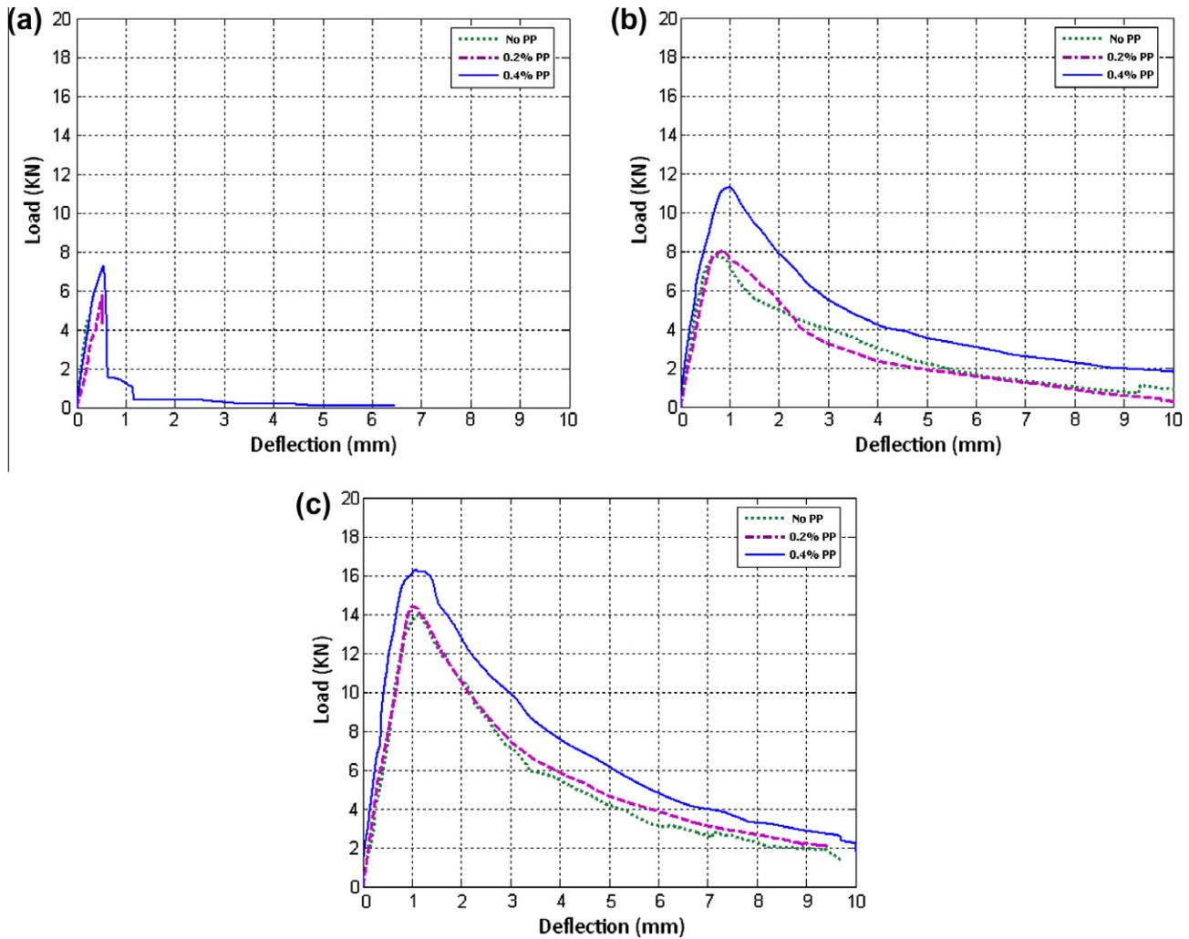
Fig. 2. Flexural behavior of concrete specimens: (a) steel fiber = 0%, (b) steel fiber = 0.5%, (c) steel fiber = 1%.
