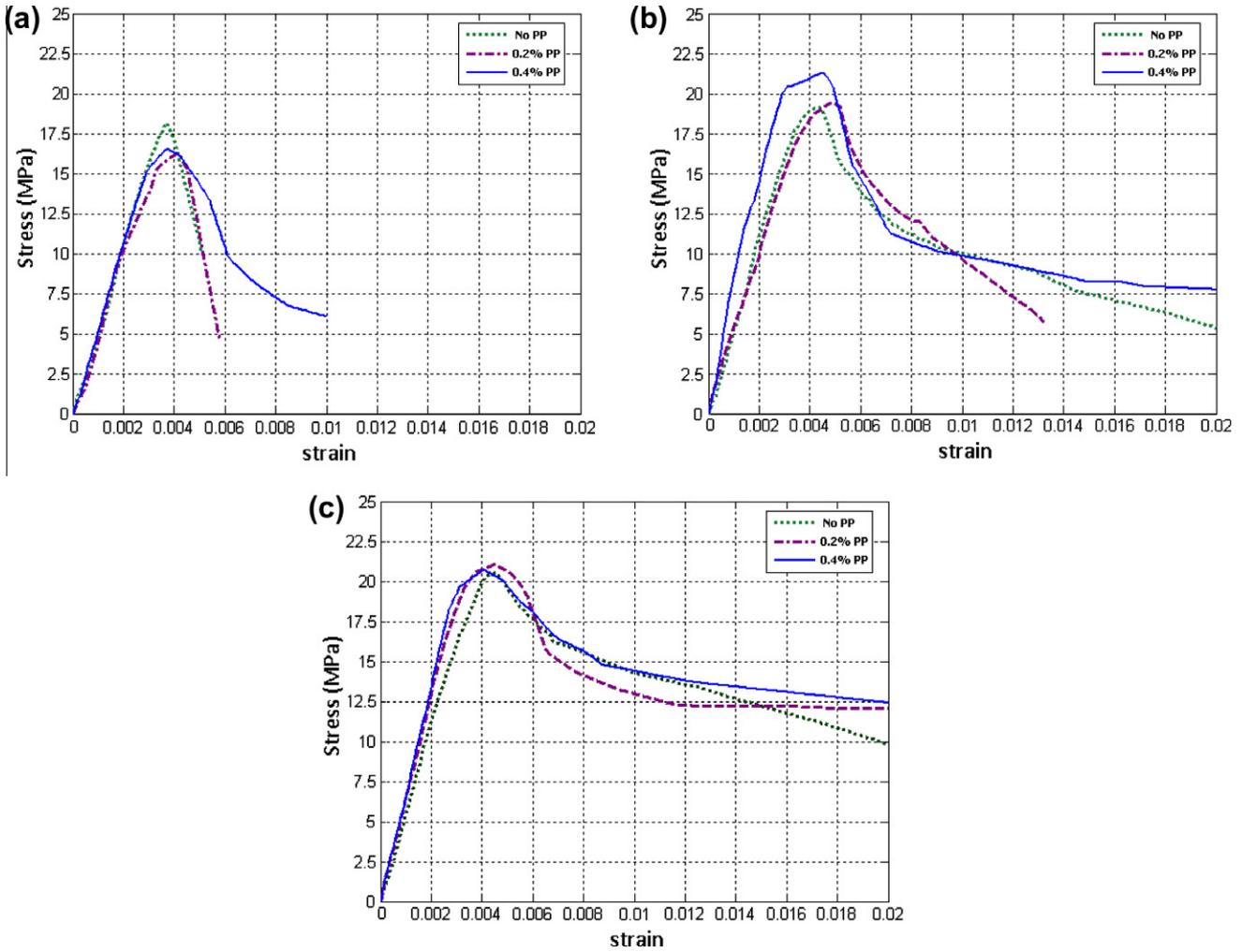
Fig. 1. Compressive behavior of concrete specimens: (a) steel fiber = 0%, (b) steel fiber = 0.5%, (c) steel fiber = 1%.
